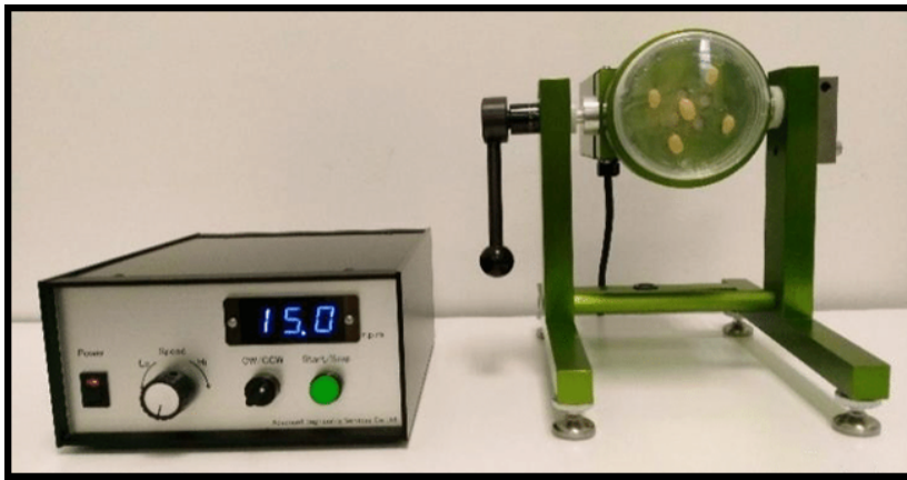
Figure 2: 2D clinostat. Image source: Researchgate scientific image library
